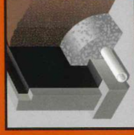
Drain tile and gravel system
